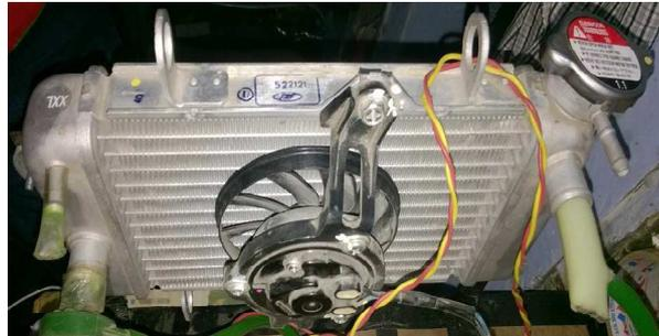
**Figure 2: Radiator and Radiator Fan**
